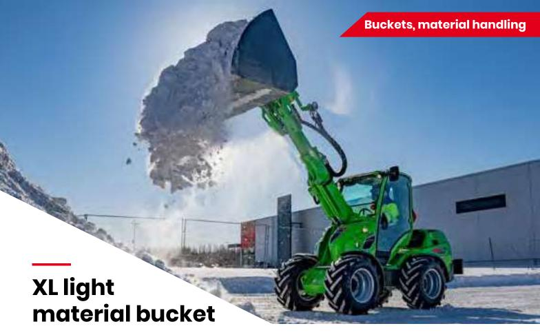
XL light material bucket is a large capacity bucket, best suited to Avant 600, 700 and 800 series. It is intended for loading and transporting of light materials like wood chips, mulch, snow etc. There are no reinforcement plates inside the bucket which would interfere when loading and emptying, and the sides open forward in a slight angle, which guarantees easy and complete emptying of all kinds of materials and in difficult conditions also.
