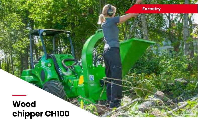
Wood chipper CH100 is a compact and robust disc chipper which Robust and compact disc chipper, works also on Avant 200 series 2 and 400 series. With it you can chip branches and small trees up to 100 mm diameter - an ideal tool for chipping wood in smaller scale. Two knives and an anvil take care of chipping and feeding. Wood feeding is manual.
