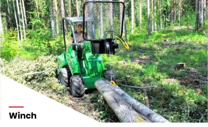
The Avant hydraulic winch enables towing of all kinds of objects (e.g. logs, poles, boats) from places where you cannot drive with the machine.
