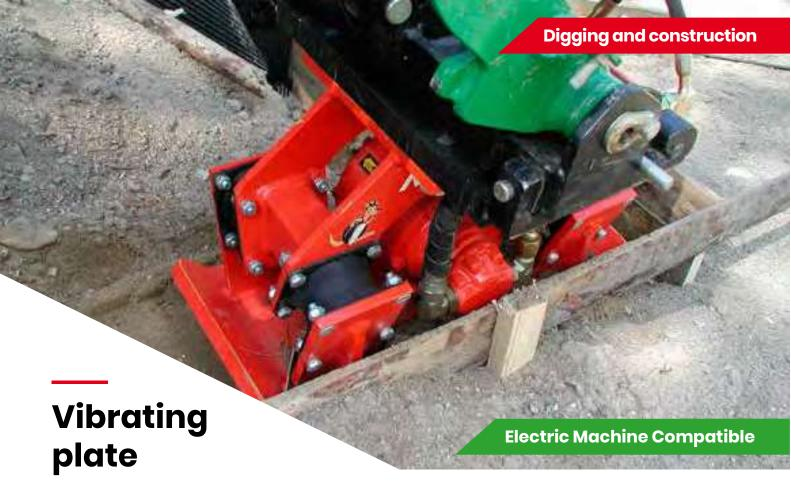
Vibrating plate is destined for earth compacting and is easy to attach to an Avant. Compacting is easy and safe with the vibrating plate connected to Avant's quick attach plate – the operator is not exposed to vibrations or excessive noise.
