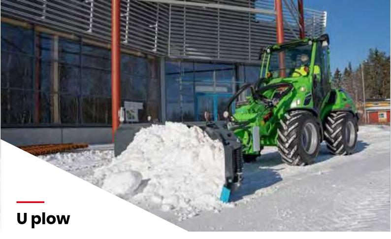
U plow is a professional tool for fast and efficient snow removal. It consists of a 1,83 m wide main blade and two side blades which can be turned ± 85° hydraulically. This allows access through narrow gates and yards, and on the other hand the max. 3 m working width with the side blades extended guarantees fast cleaning of larger areas. Collecting and pushing of large amounts of snow is also easy with the side blades turned into "U" position.
