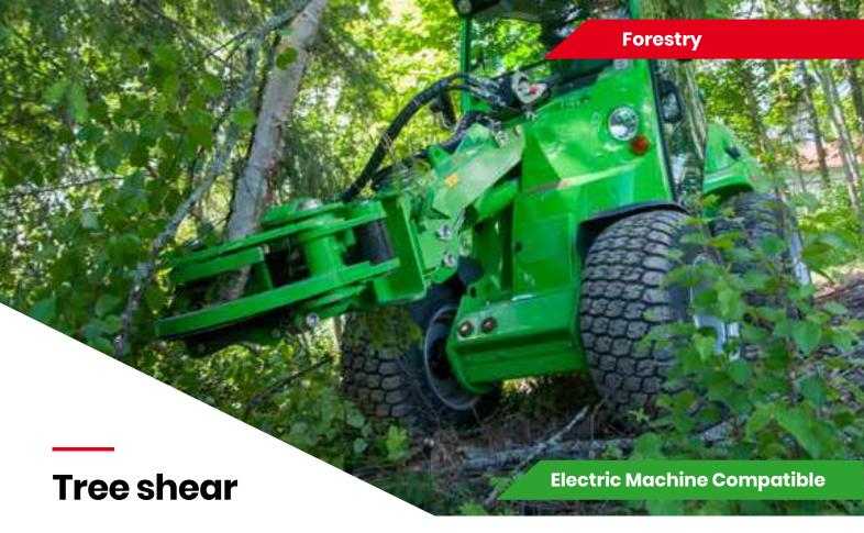
Avant tree shear is an efficient and useful tree cutter, intended for forest thinning, tree clearance and similar jobs where smaller trees need to be cut. The strong grapple takes a firm grip of the tree trunk and a hydraulic cylinder pushes the cutting blade against the trunk and cuts it. The tree is then easy and fast to move away with Avant. If needed, the cutting blade can be turned 180 degrees to point backwards. This means it doesn't cut and the unit can be used as a grapple only.
