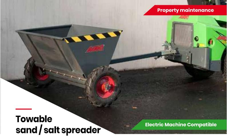
The towable sand / salt spreader is a very handy and economical attachment for winter maintenance of yards and walkways. Power to the spreader shaft is taken mechanically from the wheels. Wheels are equipped with a clutch which allows transporting
