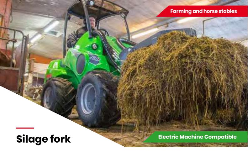
A robust silage fork equipped with a powerful hydraulic cylinder, can be fitted on all Avant loader models. The strong blade type pins of the grapple penetrate into all types of feed. The fork has replaceable lower tines made of reinforced steel. The grapple goes up to vertical position and this, together with the powerful cylinder enables easy grabbing e.g. on a round bale.
