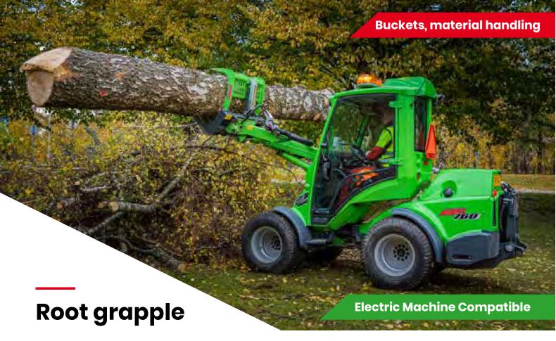
The root grapple is widely used in the tree industry, and it works also in other jobs where different types of debris needs to be handled. It is equipped with the same grapples as the demolition grapple buckets, but the bottom part is made of strong steel bars. This allows:
