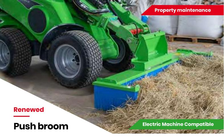
The updated push brooms feature stronger bristles and a new layout: the broom consists of individual brush strips installed in five rows, which means they can be easily replaced if necessary.
