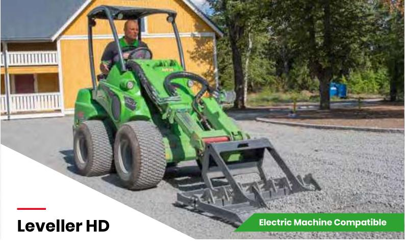
The HD leveller is an incredibly useful and efficient attachment for quick levelling of uneven ground, mulch, yards, driveways etc. It is most commonly used in:
