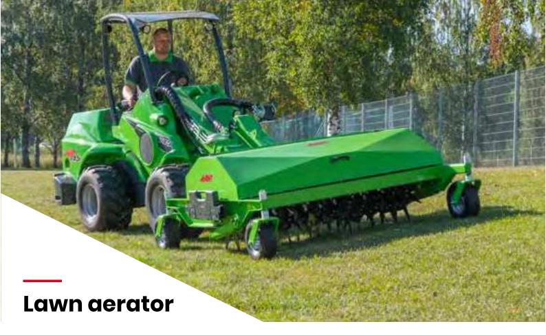
Lawn aerator is designed to create holes in the lawn surface which encourages free movement of soil. This helps to improve the circulation of air in the soil which is vital for a healthy lawn. Avant aerator is completely mechanical – when driving forward with the loader the knife type blades on the aerator shaft turn and make holes in the lawn.
