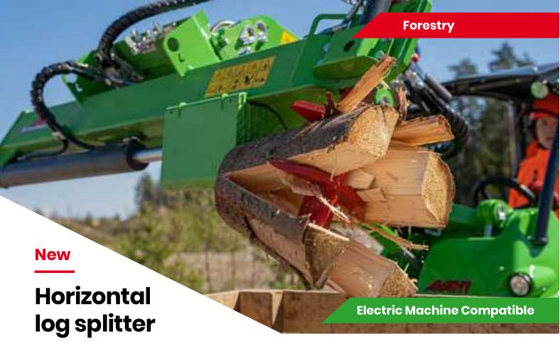
Horizontal log splitter is the most economical and simple way to make firewood with Avant. It mounts on the attachment coupling plate of the loader and is operated from the driver's seat. Splitting happens by picking up the log with the splitter and pushing it against the splitting wedge. The log can also be held with the splitter and transported to desired place for splitting.
