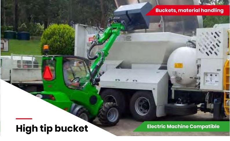
High tip bucket is the right choice when you need to reach higher and longer. The bucket is equipped with a hydraulic cylinder that pushes and tips the bucket over its front edge, which gives considerably more tipping height than with a normal bucket.
