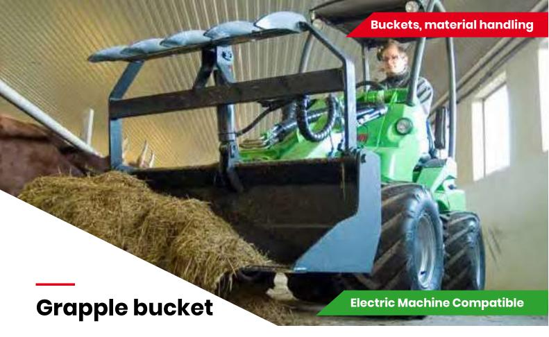
Grapple bucket combines a normal bucket and a grapple and is therefore suitable for a multitude of jobs. It can be used for transporting and loading of branches, wood chips, compost, straw, manure, construction waste etc. It can also be used as a normal bucket with the grapple in the upright position.
