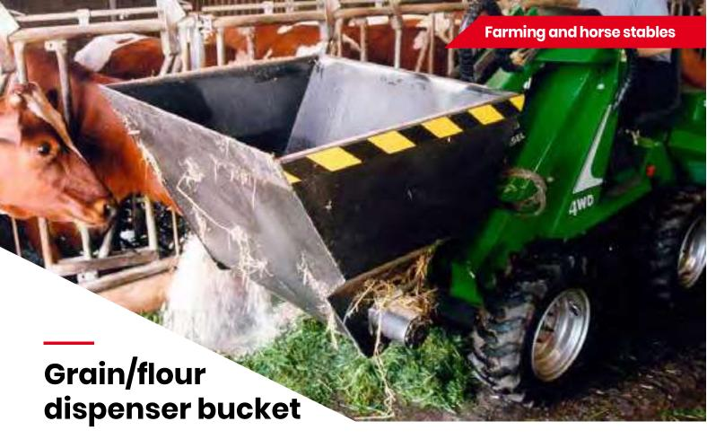
Avant grain dispenser is a 300 l bucket equipped with a hydraulic Easy distribution of flour, crushed motor and a Ø 200 mm screw, destined for distribution of flour, crushed grain etc. The bucket is available in two versions: with discharge either to the right side or to the left side.
