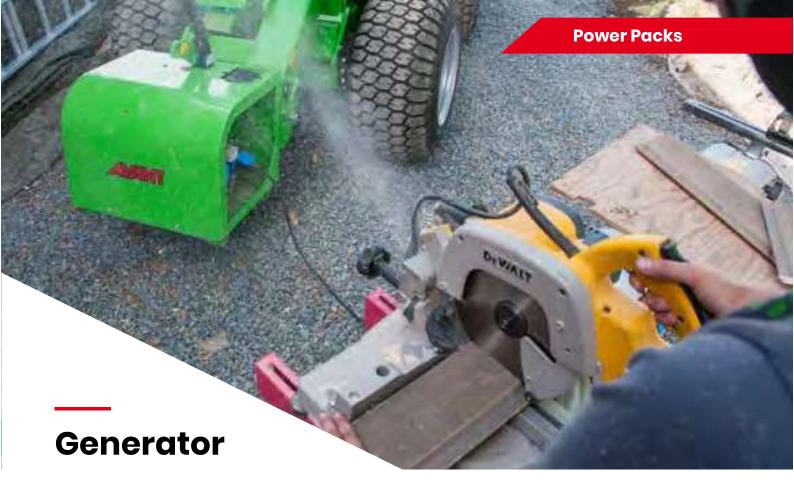
Make electricity with Avant! - The generator is equipped with Source Make electricity with Avant in 1x400V and 2x230V outlets. Generator can be used as a power source for power tools and small electrical appliances in places where net current is not available. High quality generator also guarantee electric current supply during power outages.
