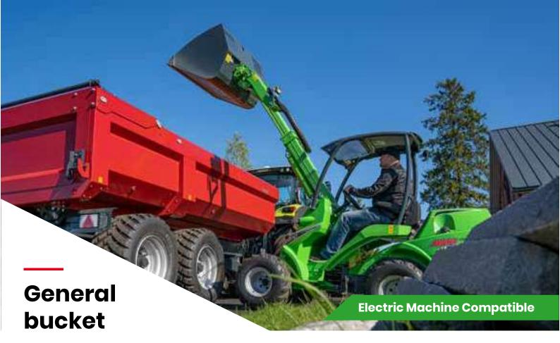
Avant general buckets are designed so that the operator can see the front edge of the bucket from the driver's seat, which means quick and easy loading and emptying. There are no reinforcement plates inside the bucket which would interfere when loading and emptying, and the sides open forward in a slight angle which guarantees easy and complete emptying of all kinds materials.
