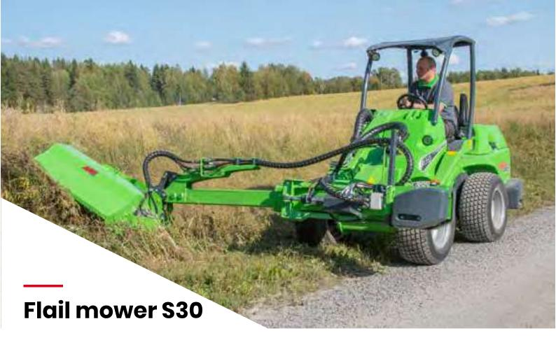
The 1200 mm flail mower with S30 quick attach bracket mounts only on the hydraulic side arm A448736. It cannot be mounted on the attachment coupling plate of the loader or on the A431070 S30 mechanical side arm - and on the other hand the normal flail mowers A36730 and A36015 cannot be mounted on the hydraulic side arm.
