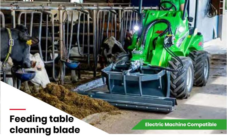
This cleaning blade is specially designed for clearing the cattle feeding table before distributing new silage to the table. The cleaning blade can be mounted by driving the silage fork into the blade, no need to get out of the driver's seat which speeds up the cleaning process, because no attachment change is necessary. The cleaning blade has a rubber lip on the lower surface that ensures good cleaning result.
