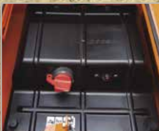
Battery cut-off switch
