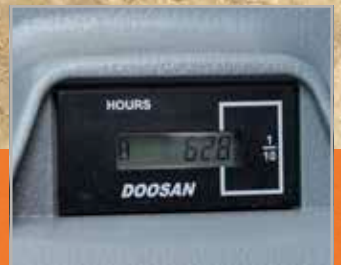
Hour meter (from ground level)
