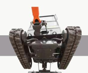
**Undercarriage:** Reinforced and expandable undercarriage from 980 mm to 1360 mm.
