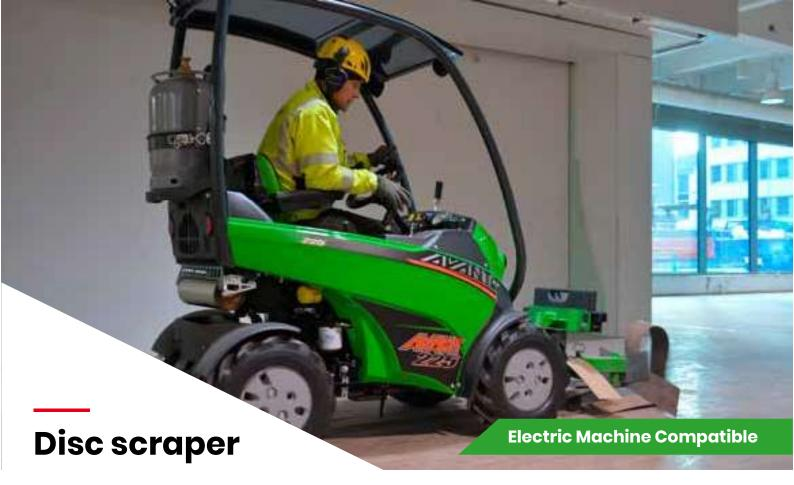
Disc scraper is an excellent and cost efficient tool for removing of carpet and floor tiles in demolition and refurbishing jobs. The durable disc takes off old carpet and tiles quickly and efficiently.
