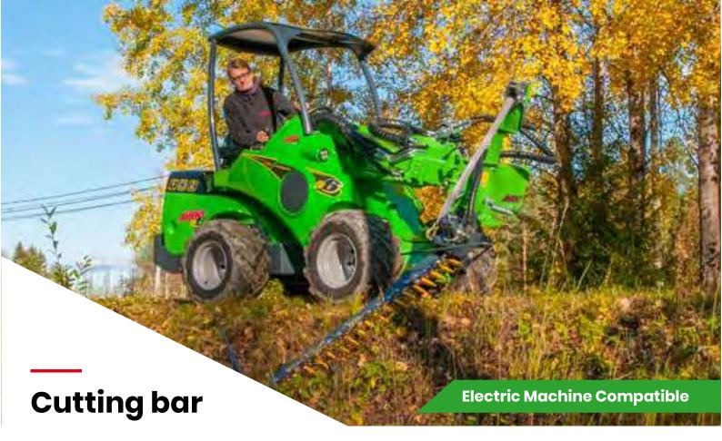
An uncomplicated cutting bar for mowing of hay, grass and Robust and economical long hay trimming of bushes and hedges. Thanks to the side mounting and angle adjustment below ground level mowing of slopes is also possible. Guide plates under the bar support the cutting blades Cutting angle adjustment below when mowing.
