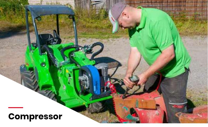
Makes it possible to have compressed air anywhere you go. Creates max. 400 l/min air flow @ 8 bar pressure. Can be used for running power tools and, for example, filling of large tyres in places where electric current is not available, and for cleaning of big machines like combined harvesters etc.
