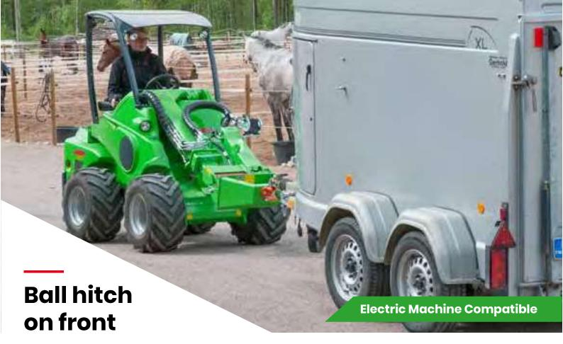
An easier way to move trailers, trailer mounted work platforms, boats on trailer etc. on yards. Thanks to the perfect vision to the ball hitch it is very easy to couple a trailer by just driving the ball under the trailer and locking it in the coupling by lifting the boom of the loader.
