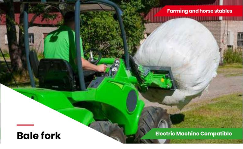
With the round bale fork transporting and lifting of bales is easy and safe. Square bale fork makes it easy and safe to transport and lift unwrapped square bales.
