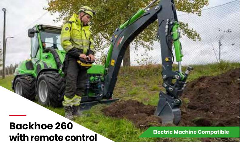
Avant backhoe 260 is now available also with radio remote control (remote control cable is also included). It allows the operator to stand next to the unit when digging and have a perfect, unrestricted field of vision to the work area. This is very useful for utility jobs, cemeteries and similar places where space is limited and exceptionally exact digging with total visibility is necessary.
