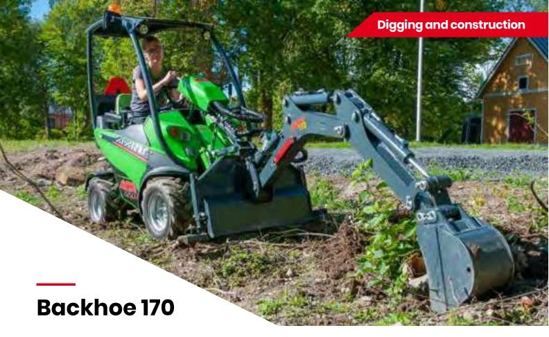
Avant backhoe 170 is a compact digging unit, intended mainly for Avant 200 series. The main focus in design was user friendliness and straight forward construction. Backhoe 170 is a small backhoe, which is at its best in tight situations where space is limited.
