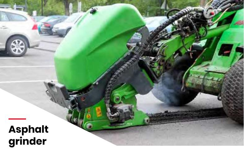
The strong and efficient asphalt grinder (also called cold planer) is an ideal attachment for asphalt road and pavement repairs and utility jobs. It grinds away the asphalt surface up to 80 mm depth, making repair of potholes, utility cuts, small overlays and edge repairs fast and easy. Different types of teeth are available for grinding of asphalt or concrete.
