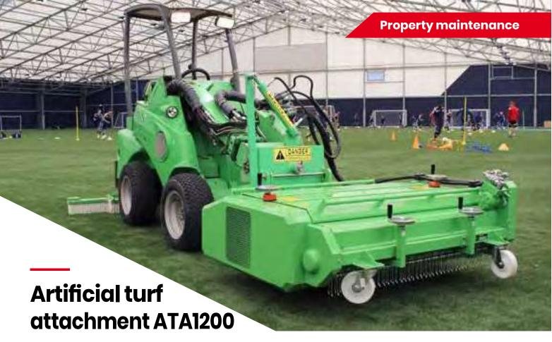
The artificial turf attachment ATA1200 is made for professionals. It Rotating main brush cleans, filters & returns the infill in a single pass. The fully hydraulic system powered with Avant performs the cleaning tasks efficiently, economically and with very low impact footprint in all artificial surfaces.
