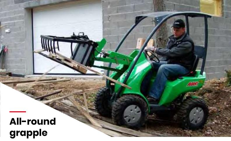
This versatile tool can be used for lifting and transporting of many different types of materials which cannot be handled with a normal bucket or pallet fork. The grapple is equipped with a hydraulic cylinder in the upper grapple part and it opens all the way up in vertical position. This, together with the pressing force of the cylinder, gives excellent loading and handling capabilities. Total width is 900 mm - this allows traveling through narrow doorways and working in small spaces.
