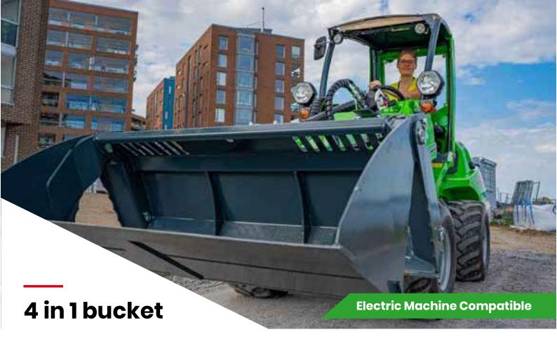
Efficient multi purpose bucket - can be used as a normal bucket as well as a dozer blade, leveler or a grab. The front part of the bucket opens with 2 hydraulic cylinders, located on the back side of the stumps etc. Another benefit of the opening bottom is that the bucket can be emptied at a higher level by opening the bottom instead of tipping the bucket edge down.
