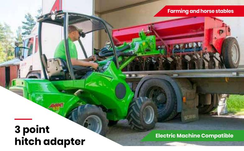
With the 3 point hitch adpater it is possible to move agricultural attachments with Avant, for instance for storage, cleaning etc. This can be practical especially when space is limited and handling with tractor is difficult. Also the trailer ball hitches can be mounted on the 3 point hitch adapter.
